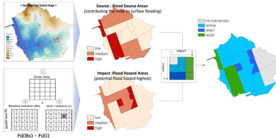
• (Source) Runoff contributions of each sub-catchment is analyzed by repeatedly executing a precipitation-omitting model
